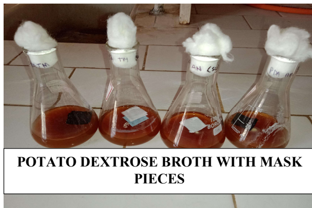
Fig-3: Biodegradation of mask using artificial microbial method
