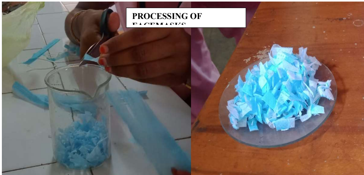
Fig-1: Processing of surgical Mask
