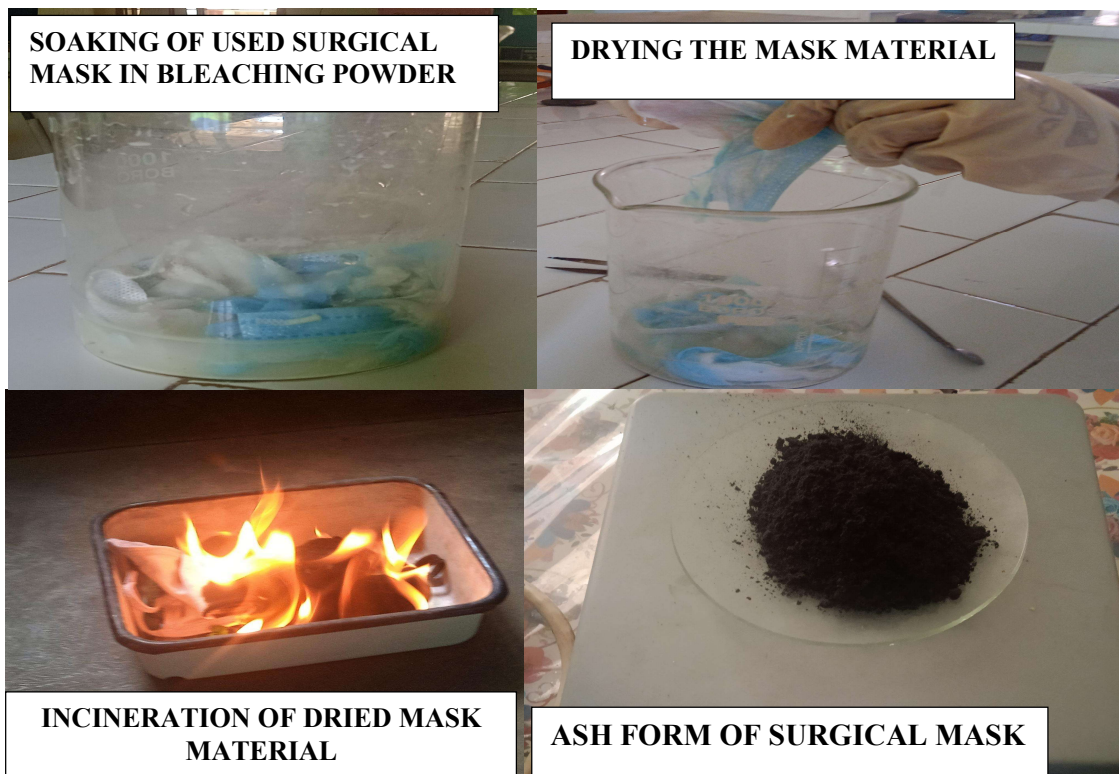
Fig-6: Processing the surgical mask to make into ash form
